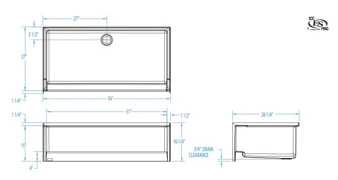
FEATURES Ibs Dimensional Tolerance ± 3/8". Dimensions needed for site preparation should be measured from the unit. Aquatic assumes no responsibility for preparatory work.
